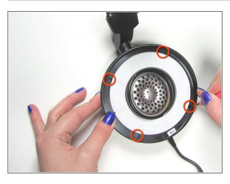
Remove all four 1cm screws on the inside of the headphone using a #1 Phillips head.
