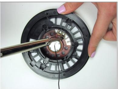
Connect the new red and yellow wires by re-soldering the wires using the soldering iron. If you need assistance, reference <u>How To Solder and Desolder Connections</u>.
