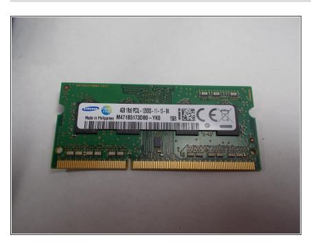
The RAM is removed and ready to be replaced.
