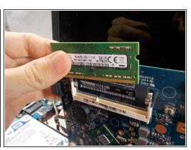
In order to remove the RAM, push both of the clips outward and the RAM chip will easily slide up and out.
