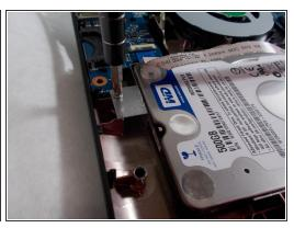
Using a Phillips #000 screwdriver, remove the five 1.2mm screws that hold the hard drive in place.
