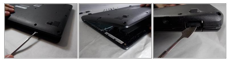
• Pry around the edges with a spudger to remove the back cover.
