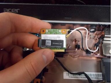
• Remove the wireless LAN card from the motherboard by unplugging the connecting wires.
