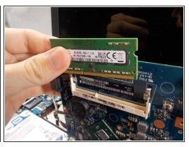
• To remove the RAM, push both of the clips outward and the RAM chip will easily slide up and out.
