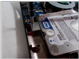
Using a Phillips #000 screwdriver, remove the five 1.2mm screws that hold the hard drive in place.
