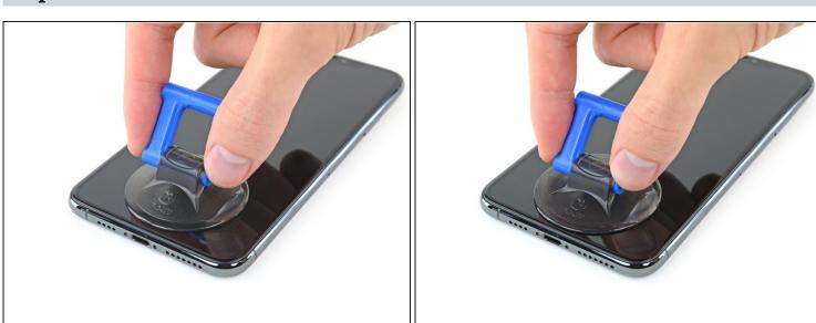
• If you're using a single suction handle, apply it to the bottom edge of the phone, while avoiding the curved portion of the glass.
