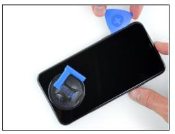
• Slide the opening pick around the lower left corner and up the left edge of the iPhone, slicing through the adhesive holding the display in place.
