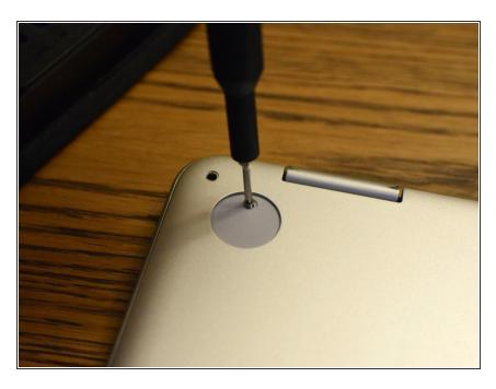
Use a #00 screwdriver to remove the 3.17 mm screws from beneath the rear feet.
