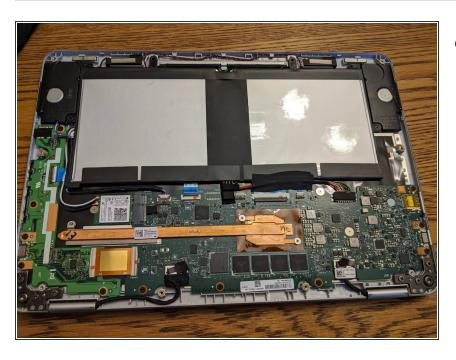
Pull away the back cover. You now have access to the battery, the write-protect screw, and other components.
