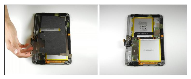
• Carefully remove the metal midframe.
