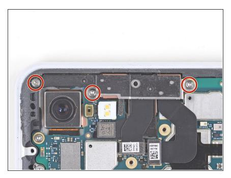
Remove the three 3 mm long T3 screws securing the front camera bracket.
