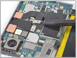
Use the point of a spudger to carefully pry up and disconnect the cameras from their motherboard sockets.
