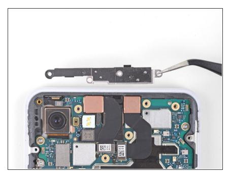
Remove the front camera bracket.
