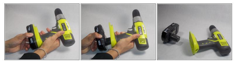
Detach the battery unit from the drill body by pressing the battery release buttons on both sides of the unit and pulling outwards.
