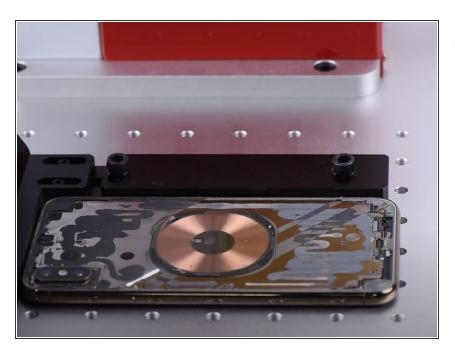
Once the back glass has been separated completely, scan with the laser light to remove residual glue on the mid-frame.
