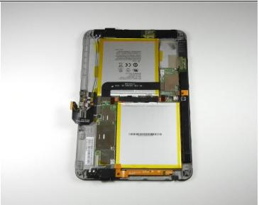
Carefully remove the metal midframe.
