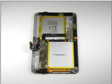
• Carefully remove the metal midframe.
