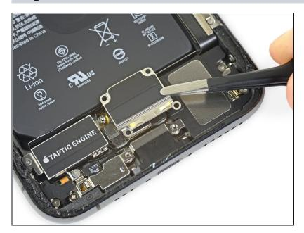
Remove the lower battery connector cover.
