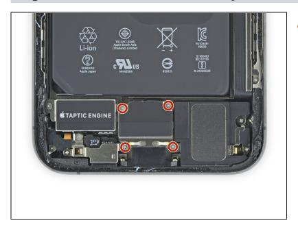
Use a Y000 driver to remove the four 1.5 mm screws securing the lower battery connector cover.
