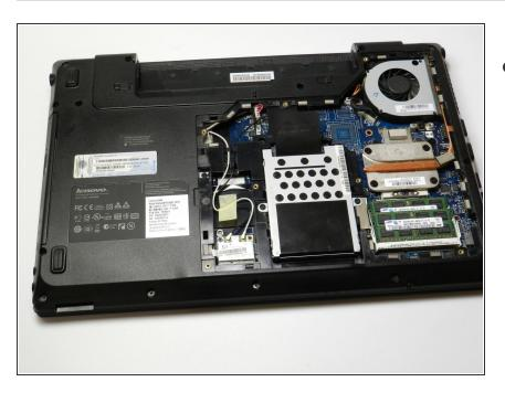
The computer should be open with many of the internal components shown. You can now access the hard drive, the RAM, and the keyboard.
