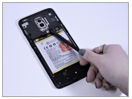
Using a spudger, gently remove the midframe and place it to the side.
