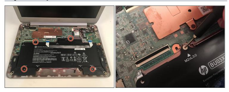
• Remove the four 3mm Phillips #000 screws holding the battery in place.
