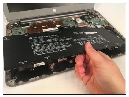
• Carefully lift the battery out of the laptop.
