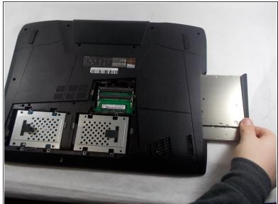
Use a spudger to pry the disc drive out of the laptop.
