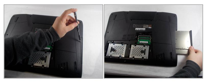
• Use a spudger to pry the disc drive out of the laptop.
