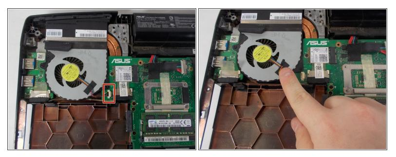
Remove the fan's power cable by pulling carefully outward towards the fan.
