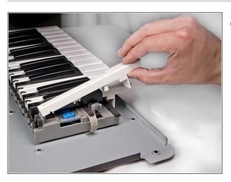
Lift the key from the front of the keyboard towards the back in order to remove it completely.
