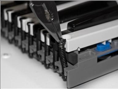
Using needle nose pliers, grip the top of the spring coil, that is holding down the key, and gently lift the spring away from the key.
