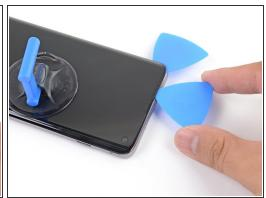
Repeat the heating and slicing procedure for the remaining display sides.
