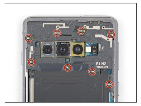
Remove the eight 4 mm Phillips screws securing the top midframe to the phone.
