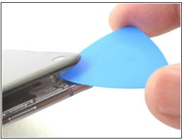
• Use an opening pick to pry open and slice through any remaining adhesive.
