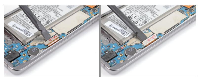
Use the flat edge of a spudger to pry up and disconnect the display connector from its motherboard socket.
