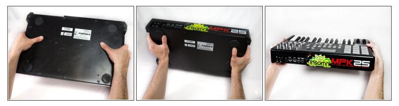
Carefully flip the device to the front making sure you secure the face plate and the chassis together.
