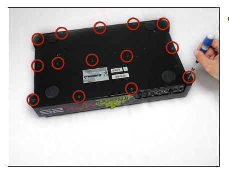
Flip the device over. Using a Philips #2 screw driver, remove the fourteen 10.3 mm black screws holding the back panel in place.
