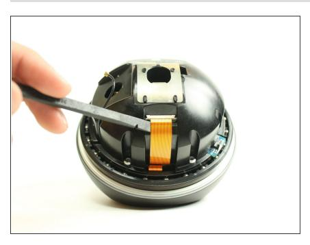
Undo the ZIF connector by prying it with a spudger.
