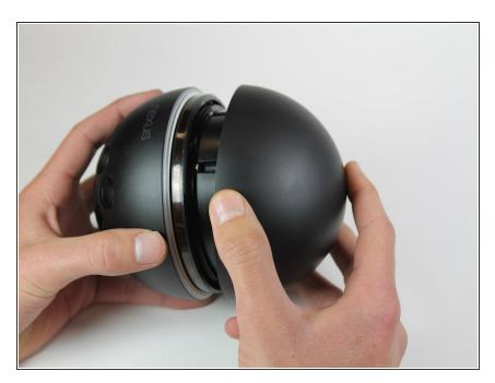
Squeeze and pull the cap to remove it from the Nexus Q.
