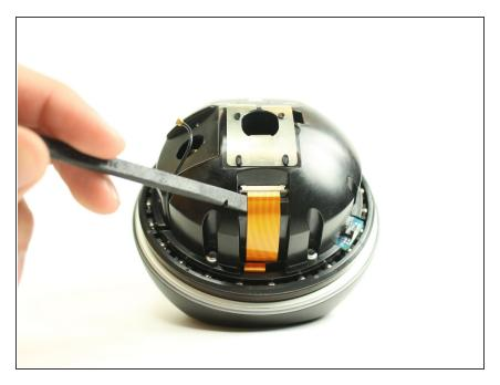
• Undo the ZIF connector by prying with a spudger.
