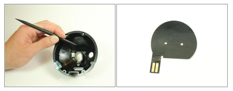
• Use a spudger to pry out the NFC antenna.
