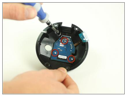
Use a T6 Torx screwdriver to undo the three 0.8 mm screws holding the inner dome daughterboard in place.
