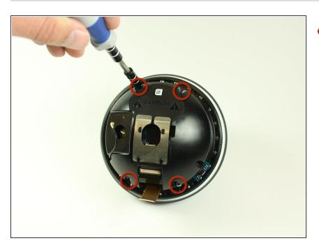
• Use a T10 Torx screwdriver to remove the four 1.3 mm screws holding the inner dome in place.
