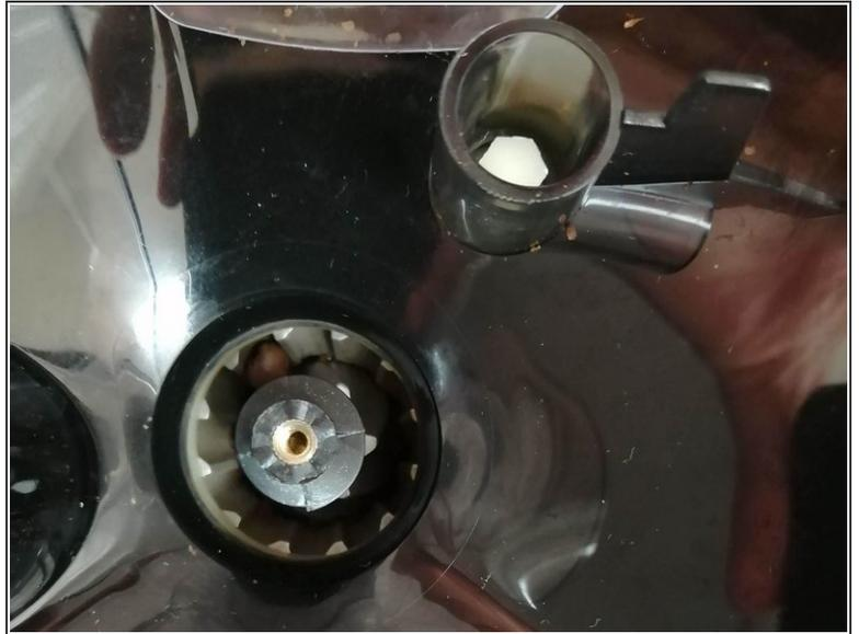
**⚠ The Hex screw must be unscrewed in the clockwise direction. Failure to do so could result in damage of the grinding mechanism.**
