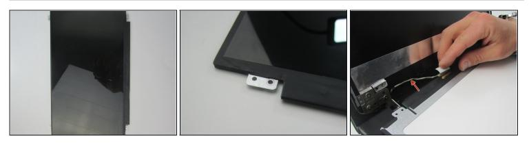
• Replace screen with new LCD screen and gently reconnect the ribbon strip.
