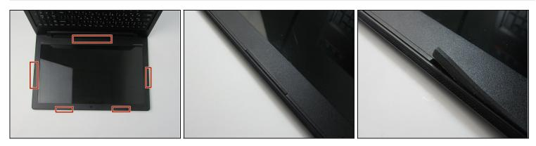
Carefully remove the laptop screen impact strips using the plastic spudger
