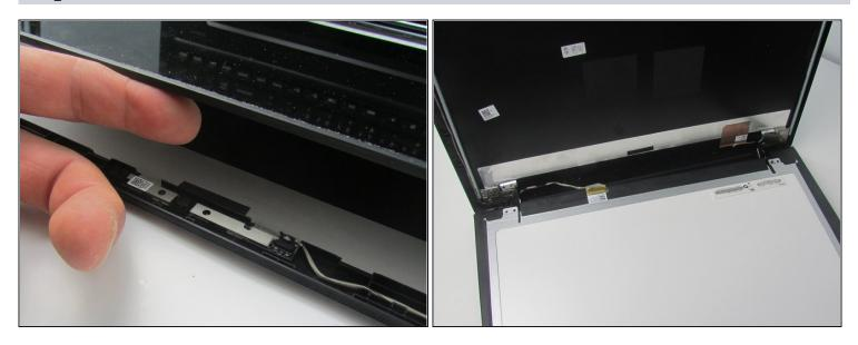
• Carefully separate screen from case, ensuring ribbon strip at the bottom doesn't become disconnected.
