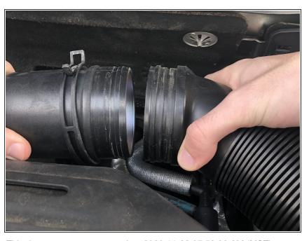
Separate the hose connection by applying a twisting and pulling force simultaneously on both ends of the connection.
