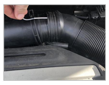
Guide the extra cleaner line through the metal hook so that it extends into the intake hose.
