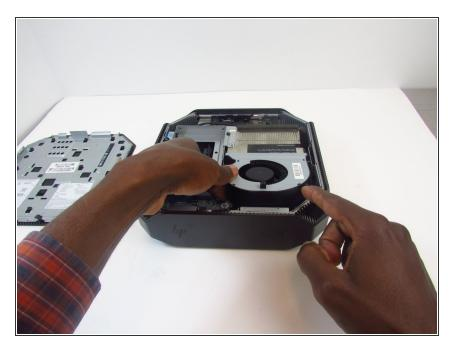
Rotate the device so the front side is facing you (the side with the power button) and locate the CPU fan.
