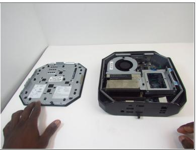
While holding the latch, lift the access panel upwards and towards yourself and set it aside upsidedown.
