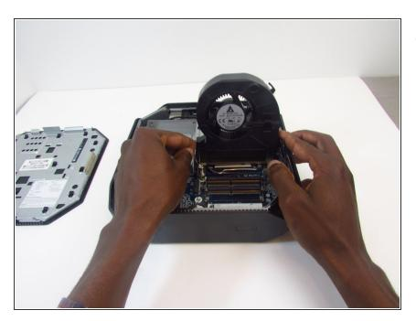
Swing the fan upward, to a 90degree angle.
