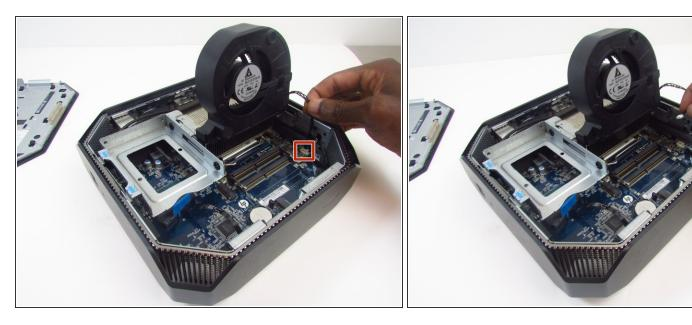
• Carefully disconnect the CPU fan by pulling out the wires from the motherboard.
