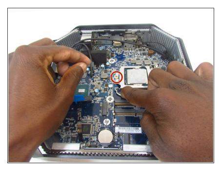
Pull the metal arm out from under the frame and lift it up. The frame should slide back from under the screw.
