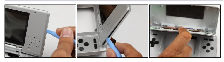
Using a plastic opening tool, pry the edges of the plastic case apart at the seam.
