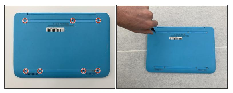
• Unscrew the seven 0.4mm screws on the backside of the laptop with the Phillips #0 Screwdriver.
