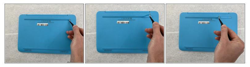
Gently peel back the two rubber strips that cover the screws on backside of the computer with the needle nose tweezers.
