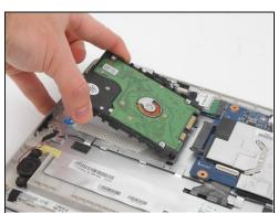
• Gently pull the hard drive towards the edge of the laptop to disconnect the hard drive from the laptop circuitry.
