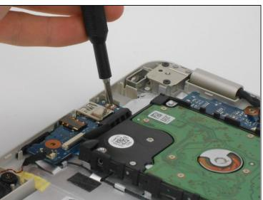
• Use Phillips #1 screwdriver (PH1 bit) to remove the 2mm screw that secures the sound board.
