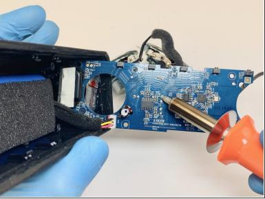
Using the soldering iron, melt the four solder connections to free the speaker wires from the motherboard.
