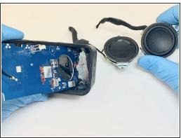
Gently pull the wires away from the motherboard to remove and disconnect the speakers from the motherboard.
