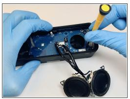
Replace the two 1mm Phillips #1 screws that hold down the motherboard.
