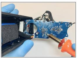
Using the soldering iron, melt the solder connections to free the speaker wires.
