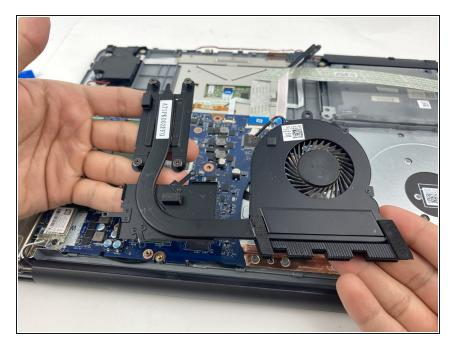
• Lift the fan and its components up and remove it.
