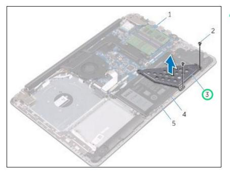
• Lift and remove the battery bracket.
