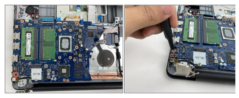
• Remove one M2.5x5 screw holding the motherboard, using a Phillips #0.
