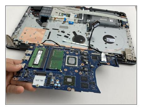
• Lift and remove the motherboard.
