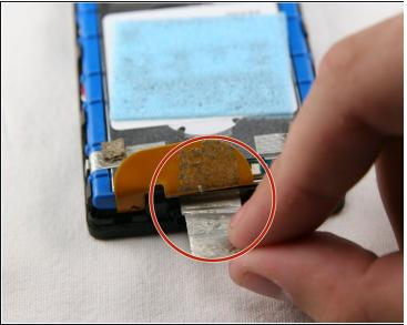
Remove the silver tape from the bottom center and the top right of the device. This allows
