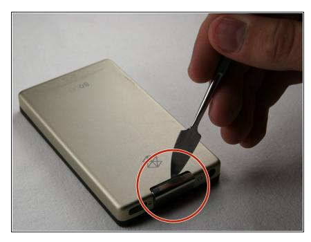
Use a metal spudger or Zune opening tool to remove the small silver plastic cap located on top of the device.
