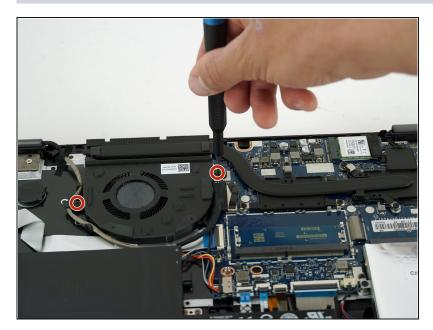
Remove the two 5 mm Phillips #00 screws that secure the fan in place.
