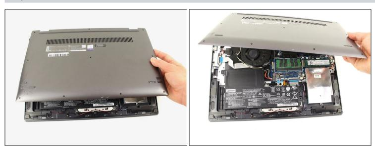
Once all the clips have been disengaged, lift off the back cover.
