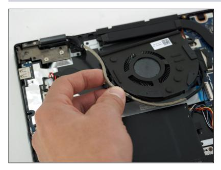
Using your hands, remove the wire that is wrapped around the base of the fan.
