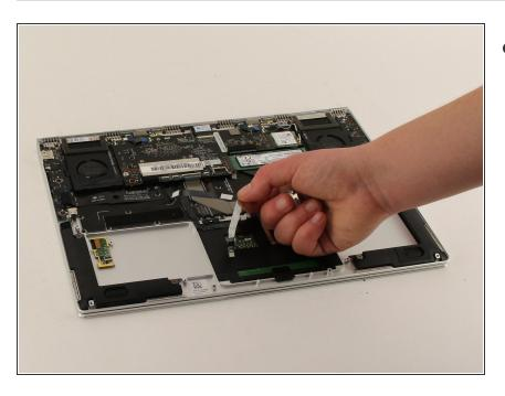
Remove the fingerprint reader from its place.
