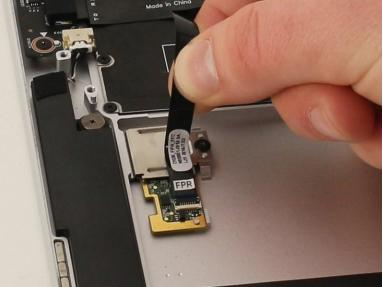
Gently pull up on the ribbon cable to detach it from the metal housing.
