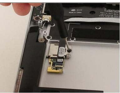
• Remove the one 3mm JIS #00 screw on the right side of the silver component.
