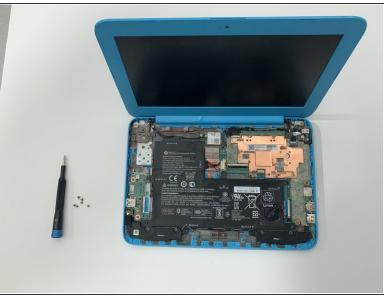
Unscrew the six 0.4mm screws surrounding the battery with a Phillips #1 screwdriver.
