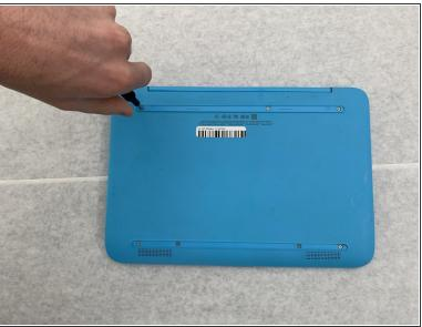
Unscrew the seven 0.4mm screws on the backside of the laptop with the Phillips #0 Screwdriver.
