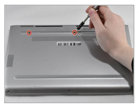
Remove the three 5.7mm Phillips #1 screws.
