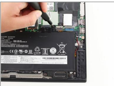
Use the Phillips #0 screwdriver to remove the four 5 mm screws that secure the battery to the laptop frame.
