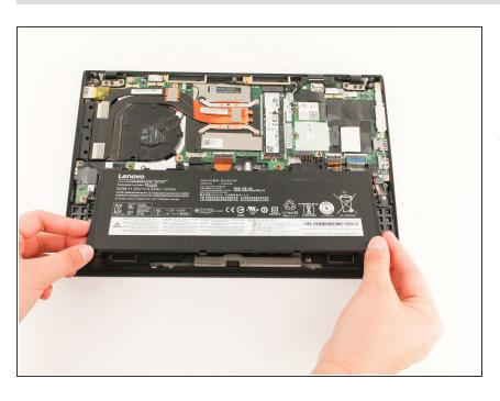
Take out the battery by lifting it from the bottom edge of the laptop, and then pulling away from the motherboard. To reassemble your device, follow these instructions in reverse order.
