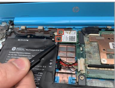
Gently pry up the two coaxial cables from the WiFi card with the needle nose tweezers.
