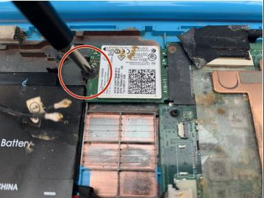
Unscrew the 0.3mm screw on the WiFi card with the Phillips #1 screwdriver.
