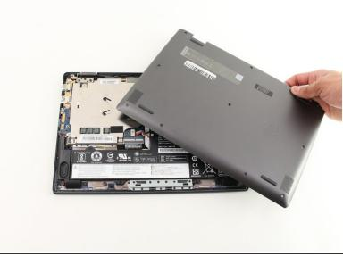
• After making sure the back panel is completely free from the body, remove the back panel.
