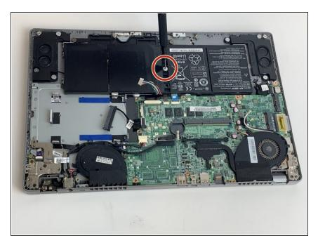
Remove the M2.5 x 3mm screw that holds down the battery using the Phillips #00 screwdriver.
