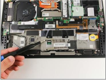
• Use a Phillips #00 screwdriver to remove the four 1mm screws that secure the touchpad to the laptop.
