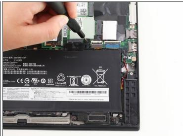
• Use the Phillips #0 screwdriver to remove the four 5 mm screws that secure the battery to the laptop frame.
