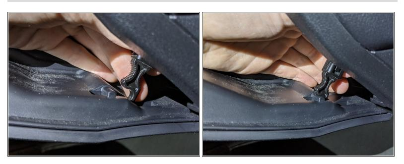
Re-clip the hook on the right side of the glovebox until it is fully engaged.
