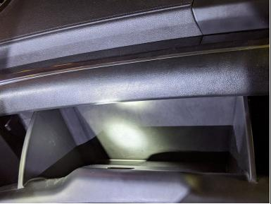
Push the glovebox up until you feel a detent where it is self supported but is not fully in the upposition.
