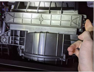
Place the cabin air filter protective cover over top of the filter until you hear audible clicks from the clasps engaging.
