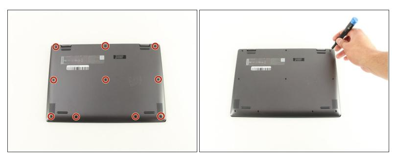
• Remove the ten screws with a Phillips #00 screwdriver.
