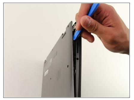
Using a plastic opening tool, make your way around the edge of the laptop.
