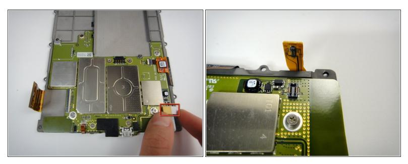
• Remove the white flex cable by gently lifting the yellow plastic connector.
