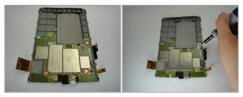
Ise a Philips screwdriver to remove the seven 3.0 mm Phillips screws securing the motherboard:
