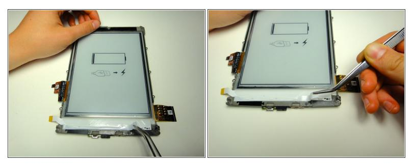
• Use a pair of tweezers to remove the white strip of tape that covers the LED lights.
