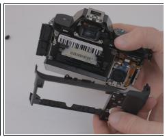
• Once the screws have been removed, unsnap and lift the rear plastic cover off of the camera.
