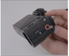
• Remove the six M1.5x4mm screws with a PH00 Phillips screwdriver.
