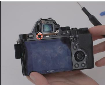
Remove the four M 1.5x2mm screws.
