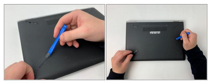
• Use the opening tool to remove the rubber feet attached to the bottom of the device.
