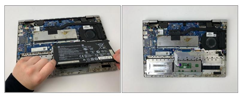
• Carefully lift from the base and remove the battery.
