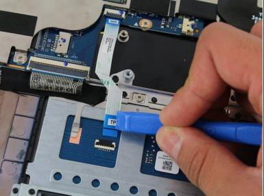
Remove the connecting wire labelled "TP" by lifting the tab with the opening tool.
