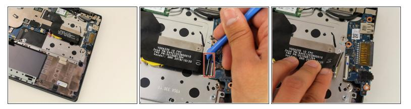
Disconnect the ribbon connector using the iFixit opening tool tool by flipping up the black flap and pulling the ribbon out.
