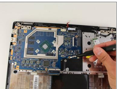
Unscrew the three 3.5 mm retaining screws from the motherboard using a Phillips #00 screwdriver.
