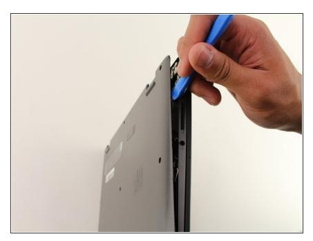
Using a plastic opening tool, make your way around the edge of the laptop.
