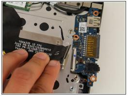
Disconnect the ribbon connector from both ends by disengaging the black latch and pulling it directly from its port.
