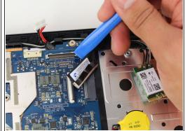
Use an opening tool to remove the connecting cables.
