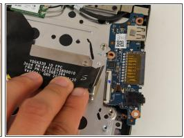
• Disconnect the ribbon connector using the iFixit opening tool tool by flipping up the black flap and pulling the ribbon out.
