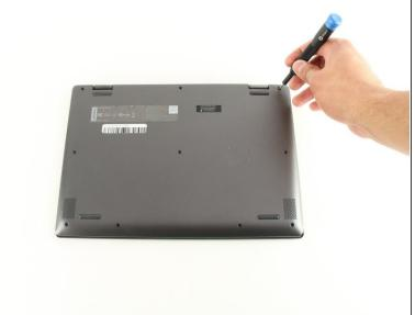
Remove the ten screws with a Phillips #00 screwdriver.
